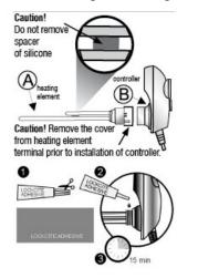
2. Screw the heating element in by means of S22 wrench, while positioning the mark on the head upwards.
