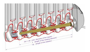
Prior to screwing the heating element in, spread the Loctite sealant (included) over the half of thread's circumference. A special silicone gasket on the head facilitates setting the thermostat housing upright. The conical gasket does not have to be tightened until resistance is felt. Using the sealant prevents unscrewing the heater when the regulator housing is accidentally hit.
