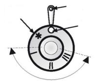
The Turbo function can be started by pressing the knob. The heater will operate at full power for 1, 2 or 3 hours.
