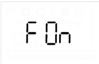
F On: Window Opening detection enabled
